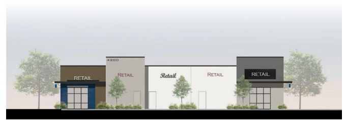
Conceptual Street Elevation Option B: Hollow Metal Doors Painted To Match Adjacent Surface
